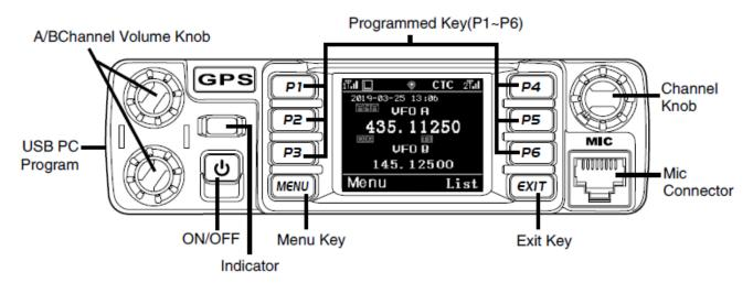
Press (Menu) key to enter the menu, turn channel knob to the Device Info and enter into the menu to check the model.
