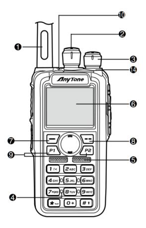
Press 7 (Menu) key to enter the menu, press very key to the Device Info and enter into the menu to check the model.
