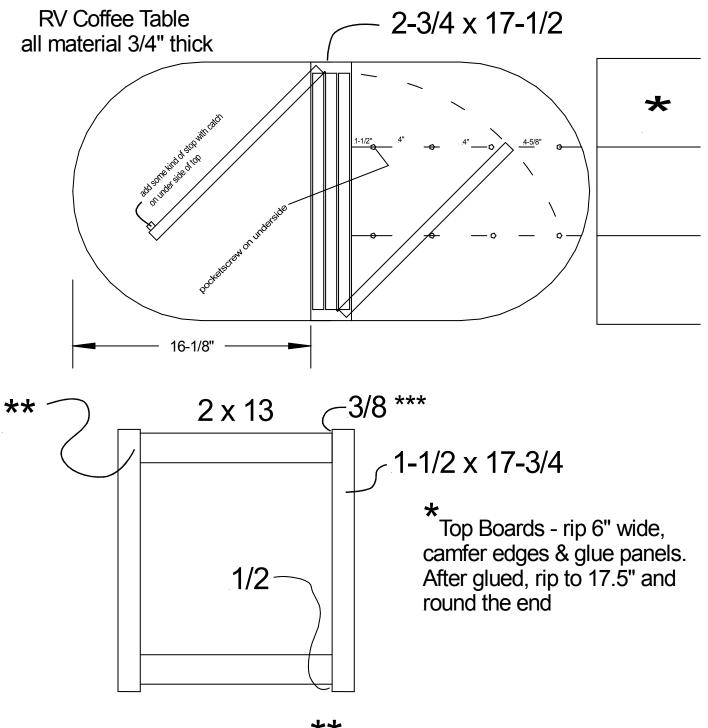
\*\* Consider camfer on edges so that the edge alignment is not as critical
